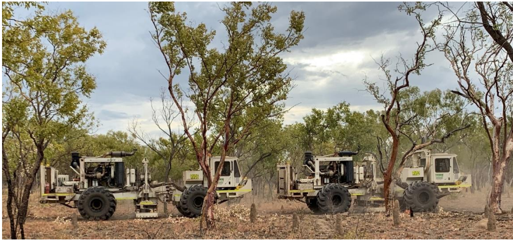
Velseis vibroseis trucks acquiring seismic data in EP187
