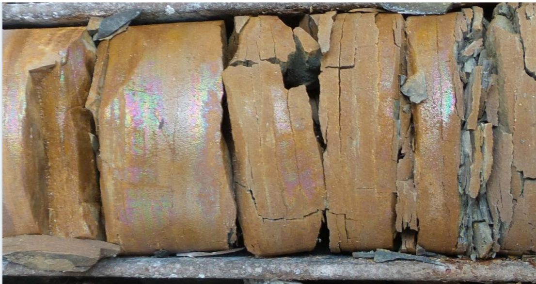
Plate 1: MD4 Core displaying the classic sheen of live oil exuding from the Velkerri shales. This core has been stored within the NTGS core library sheds in Darwin since 1993 (over 22 years) and continues to weep oil.
